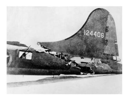
Although the tail actually bounced and swayed in the wind and twisted when the plane turned and all the control cables were severed, except one single elevator cable still worked, and the aircraft still flew - miraculously!
